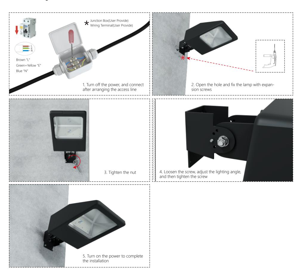
\* Note: Please make sure the power off before opertion, Installation must be performed by skilled electrician who are familiar with the requirements and proper installation methods of LED luminaire, in order to avoid damage or hazard; The external flexible cable or cord of this luminaire can not be replaced, if the cord is damaged, the luminaire must be destroyed, The light source contained in this luminaire shall only be replaced by a qualified person;
